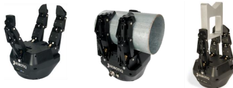
Figure 25. Adaptive gripper holding different components. (Motoman web-site, 2012)
