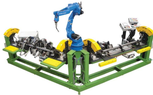
Figure 5. Two-operation welding fixture for a cross car beam. (Nash web-site, 2016)
